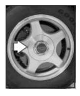
To remove the wheel center cap, use the flat end of the wheel wrench and pry them off at the pry off notch.
